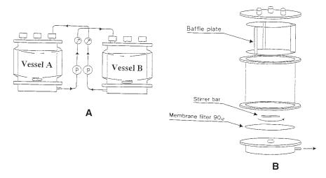
Fig. 4. Diagrams of the M-3 apparatus. (A) The experimental setup; (B) various parts of a vessel.
