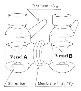
Fig. 2. A schematic diagram of the M-1 apparatus.
