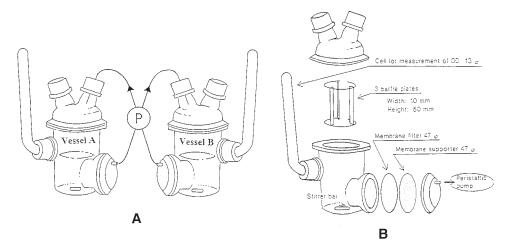
Fig. 3. Diagrams of the M-2 apparatus. (A) The experimental setup; (B) various parts of a vessel.
